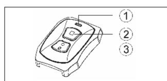
Press the Inquiry/Record Button (3) and the Photo button (2) simultaneously to enter Pairing mode
