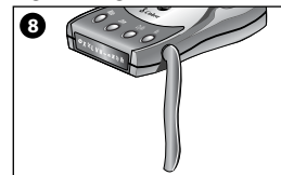
Place antenna facing towards dashboard if windshield angle prevents you from placing it upright.
