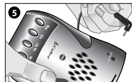
Plug power cord into detector.
