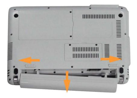
To replace the battery, slide it into the end until it clicks into place.
