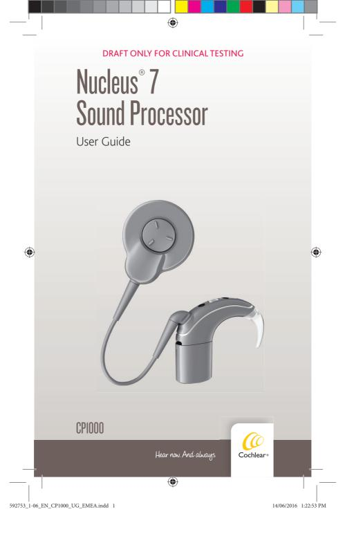
This guide is intended for Cochlear implant recipients and their carers using the Cochlear  $^{\text{TM}}$  Nucleus  $^{\text{TM}}$  7 Sound Processor (model number: CP1000). The processor works with your implant to transfer sound to your ear, and is made up of a processing unit, earhook, coil and cable, and a battery module.
