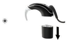
2. Pull the battery module from the processing unit.
