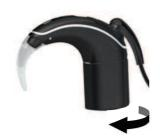
Twist the battery module as shown to release it from the processing unit.
