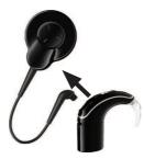
Hold the coil cable grip and firmly pull it straight out of the processor.
