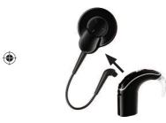
Hold the coil cable grip and firmly pull it straight out of the processor.
