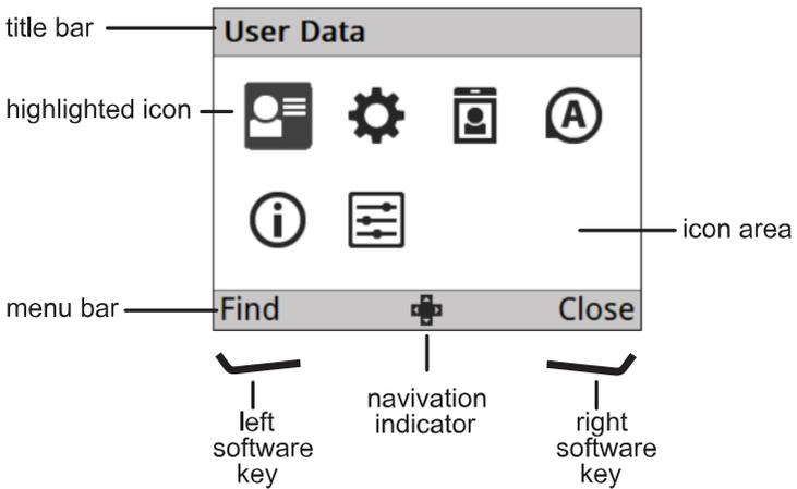
You can access the menu screen by pressing
