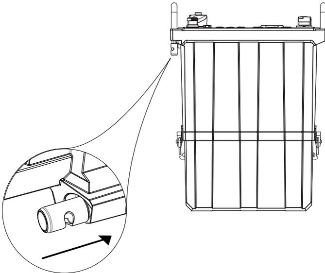
Connect the grounding wire or counterpoise lead to the grounding lug and deploy as suggested on the tactical antenna quick reference card.
