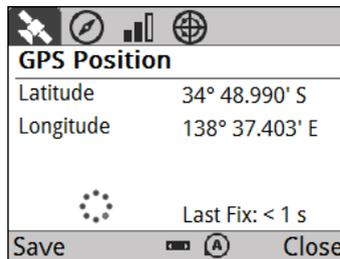
**Note:** The Sentry-H 6110-MP radio uses two Global Navigation Satellite Systems (GNSS) to calculate position information with improved accuracy and reduced time for signal acquisition.
