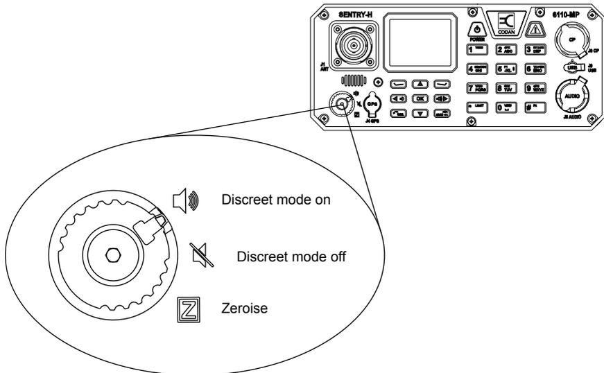
The discreet mode switch can also be configured to zeroise (erase) or lock the radio to prevent unauthorised access to the unit when compromised. By default, the zeroise function is set to prompt the user with erase or lock options.
