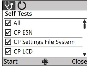
The radio will now run through all of the self tests listed on the Self Tests screen. As each test is completed, the test result will appear on the screen.
