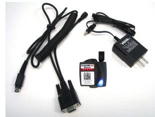
RS-232 Cable (Left) - CodeXML M3 Bluetooth® Modem (Center) - Power Supply (Right)
