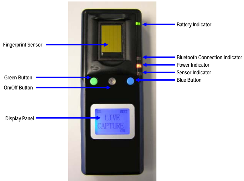
Figure 1-2 BlueCheck Capture Device Features
