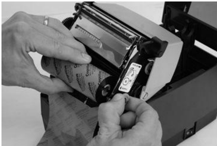
Figure 2-27. Lining up the Ribbon Supply Core Notches with the Supply Spindle Notches
