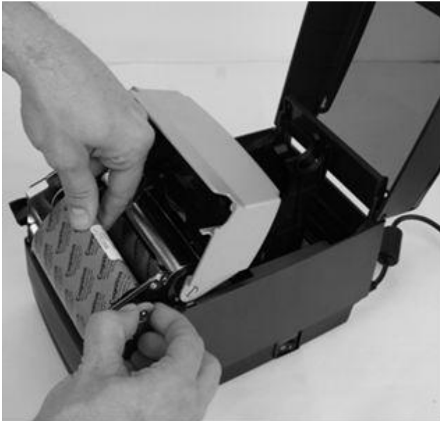
Figure 2-34. Seating the Ribbon Take Up Core Into the Take Up Spindle Notches
