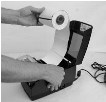
Figure 2-43a. Media Print Side Must be Facing Up for Inward Wound Media
