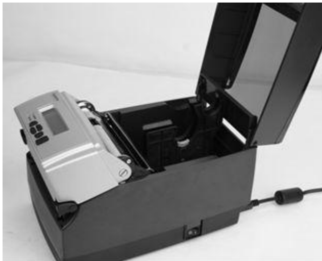
Figure 2-20. Lifting the Dust Cover
