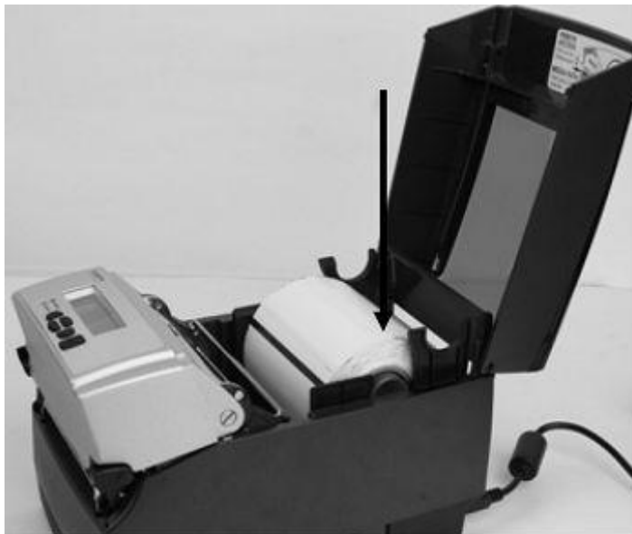
Figure 2-46. Push Down on the Right Side of the Roll to Lock the Media Guide
