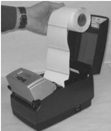
Figure 2-43b. Media Print Side Must be Facing Up for Outward Wound Media
