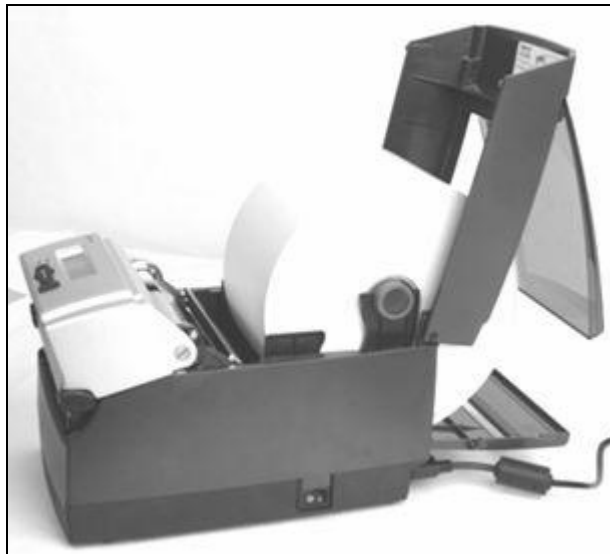
Figure 2-60. Large Media Roll in Position
