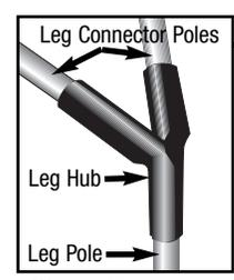
Illus. 3 Leg Hub Partially assembled frame locked into hub
