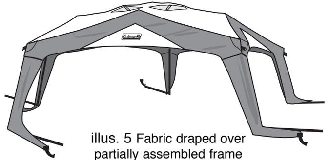
illus. 5 Fabric draped over partially assembled frame
