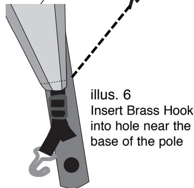
illus. 6 Insert Brass Hook into hole near the base of the pole
