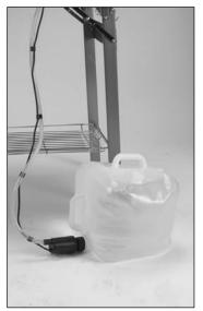
Step 2: Lay the Water Container on its side so the Pump is towards the bottom of the container.
