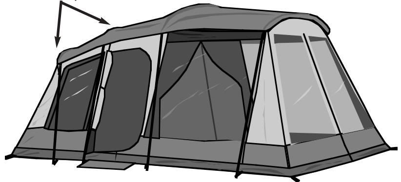
illus. 9 Tent shown completely set-up. Note the different angles of the end brace poles.
