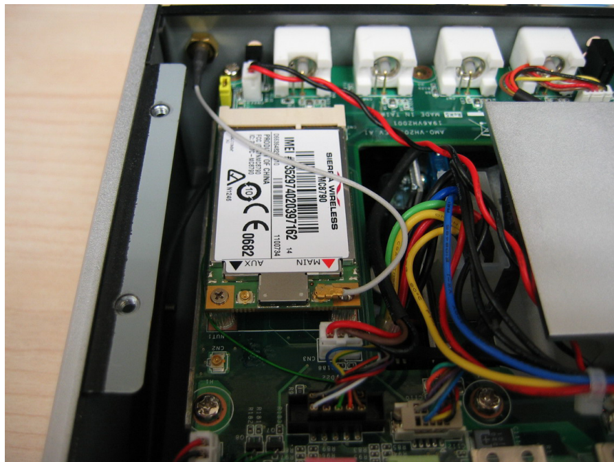
Figure 2.30 Connect the SMA Cable to the miniPCle card module
