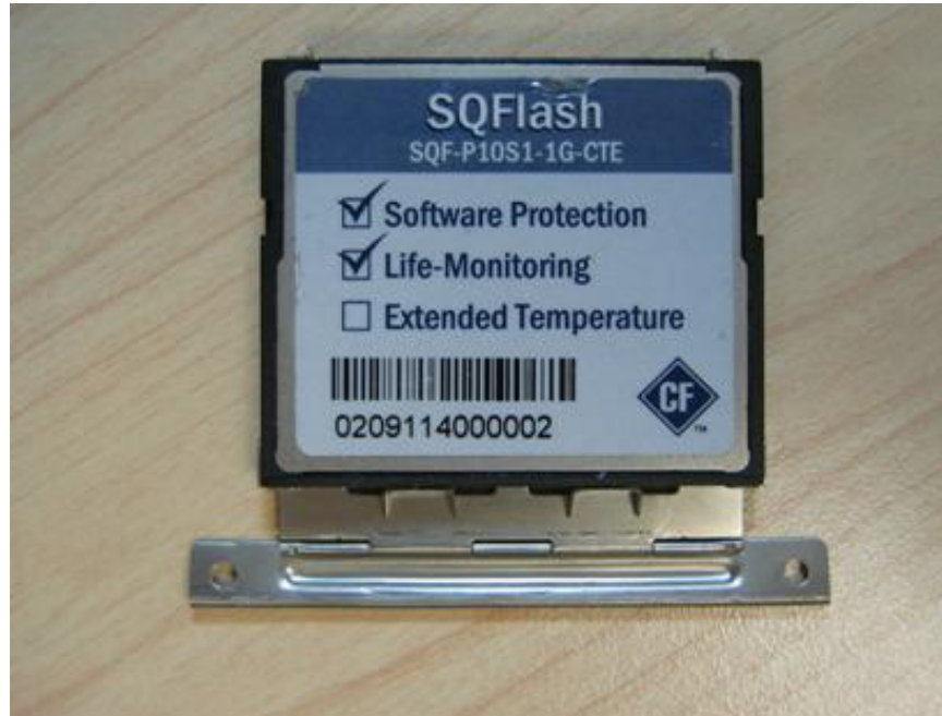
Figure 2.25 Put CF onto the CF tray
