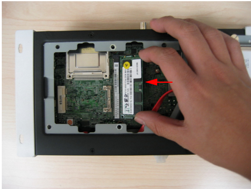
Figure 2.21 Install the memory module into the SO-DIMM socket at the bottom of the Main board
