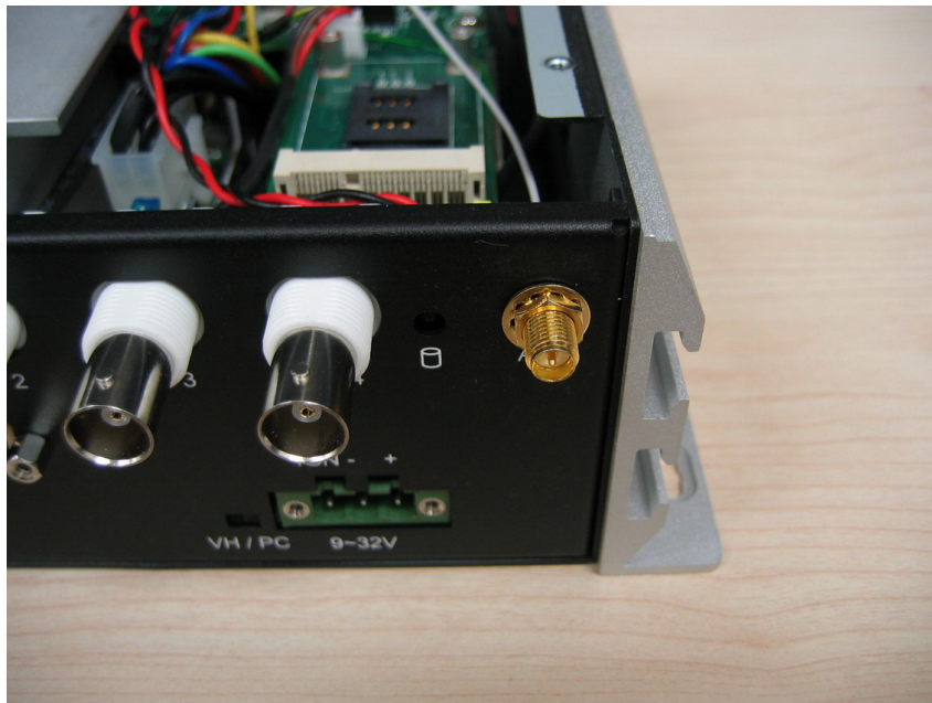
Figure 2.27 Knock out ANT hole and screw the SMA Cable into the front panel
