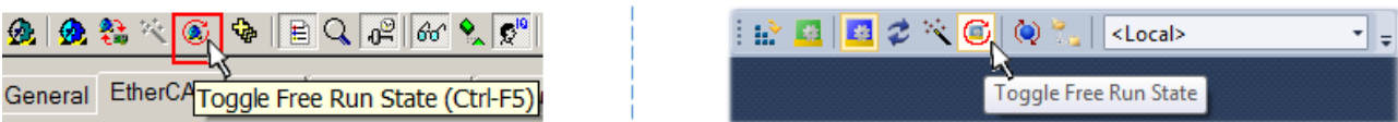
Fig. 123: TwinCAT can also be switched to this state by using a button (left: TwinCAT 2; right: TwinCAT 3)
