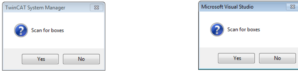
Fig. 110: Scan query after automatic creation of an EtherCAT device (left: TwinCAT 2; right: TwinCAT 3)
