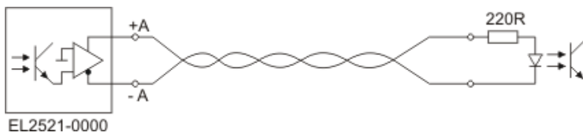
Fig. 35: EL2521-0000, direct connection to an optocoupler
