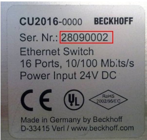
Fig. 3: CU2016 switch with batch number
