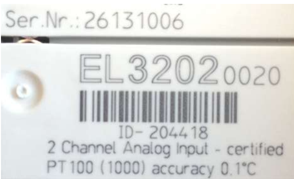
Fig. 4: EL3202-0020 with batch numbers 26131006 and unique ID-number 204418
