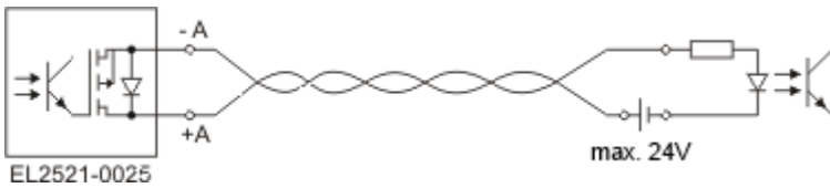
Fig. 37: EL2521-0025, wiring with external current source, logic reversal
