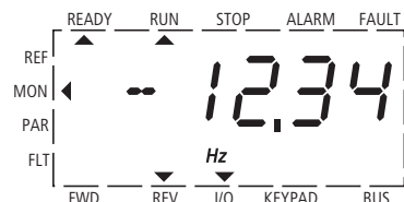
Figure 61: Operation (RUN) via control signal terminal (I/O) with left rotating field (REV) (e.g. - 12.34 Hz)
