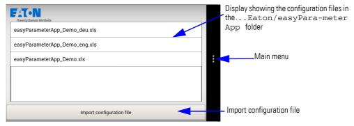
figure 11: Import menu view showing the configuration files found in the generated folder
