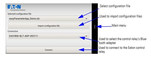
figure 9: Start page with user interface and control relay already selected
