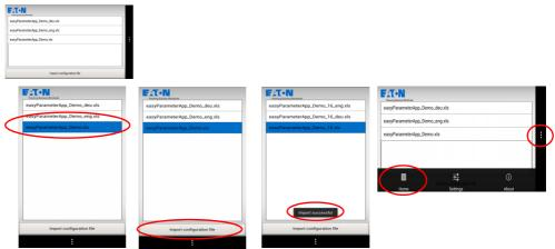
figure 23: Importing a configuration file as a user interface
