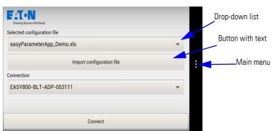
figure 6: Start page with user interface and control relay already selected
