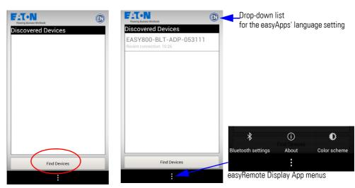
figure 2: Searching for Bluetooth adapters using the easyRemote Display App
