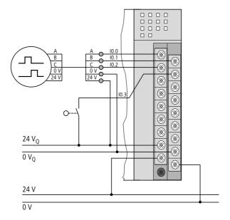
Figure 14:Connection of the incremental value encoder with a reference window switch
