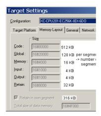
Figure 44:Segment size of the XC-CPU201-EC256k
