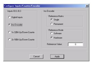
Figure 68:Incremental encoder parametric programming
