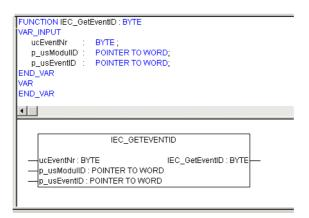
Figure 85: "IEC\_GetEventID" with declaration section function
