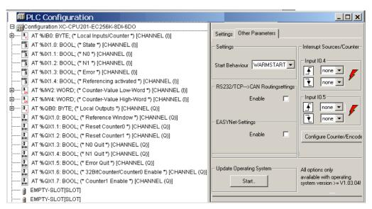
Figure 63:PLC configuration
