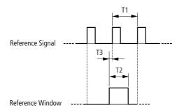
Figure 70:Relationship between reference signal and reference window
