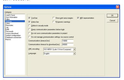
Figure 22:Setting the transfer time
