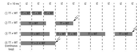
Figure 40: Watchdog active, multiple tasks with differing priority
