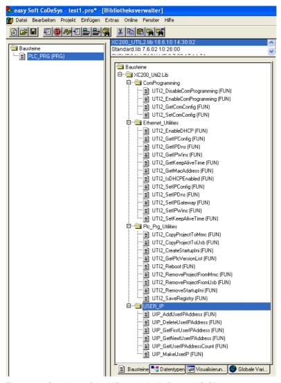
Figure 101:Overview of the XC200\_Util2.lib for the XC-CPU202
