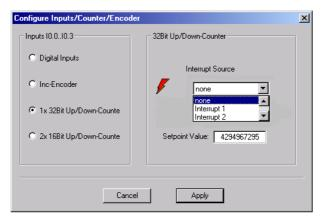
Figure 71:Parameterization of 1 × 32 Bit counter input
