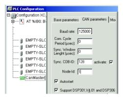
Figure 58:CAN Master: Node ID for basis communication
