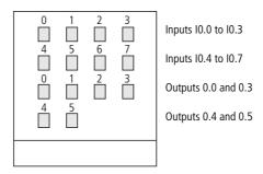
Figure 4: LEDs for the local inputs/outputs
