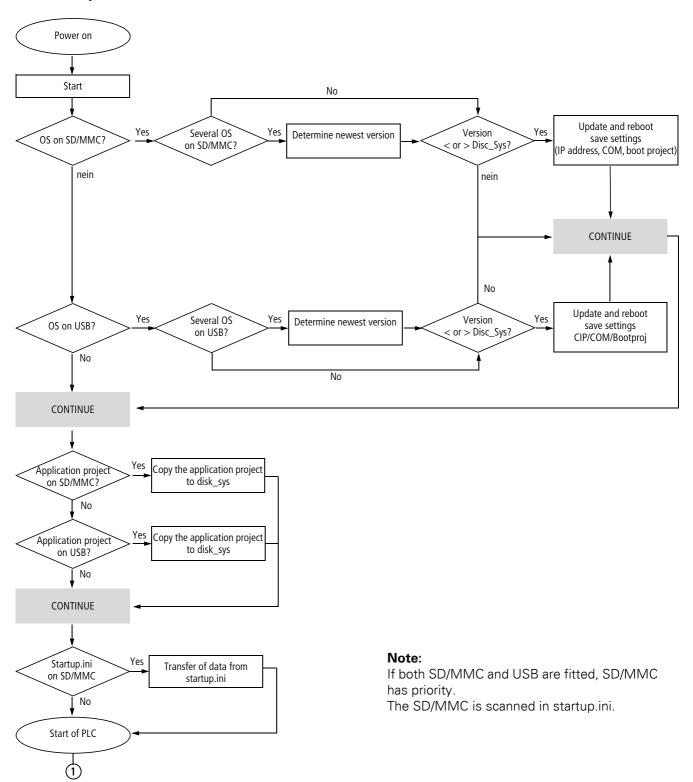
Figure 21:Boot procedure with SD/MMC and USB
