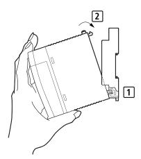
Figure 9: CPU installation
