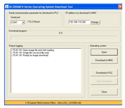
Figure 25:Download of the XC-CPU201 operating system
