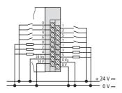
Figure 13:Connecting inputs/outputs to the central processing unit
