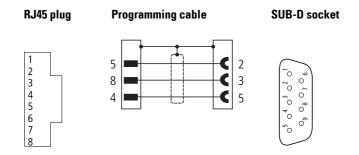
Figure 19:Pin assignment RS232 programming cable
