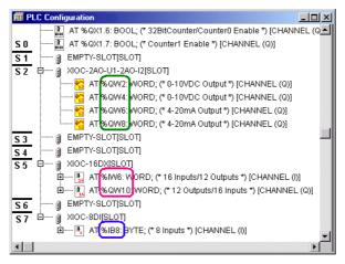
Figure 65:Configuration change by changing the modules (S0, S1, ..., S7 = slot number of the rack)
