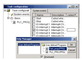
Figure 77: Allocation of Interrupt source → POU
