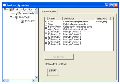
Figure 34:Assigning the POU to a system event
