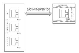
Figure 6: Connection of the XC-CPU200 with the XT-RJ45-ETH-RS232
