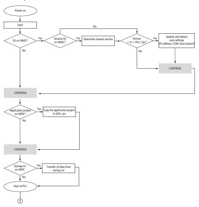
Figure 20:Boot procedure with MMC
