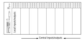
Figure 1: Layout of the XC-CPU201 with XIOC modules
