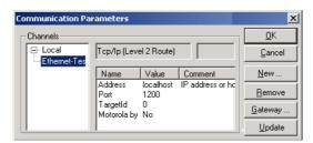
Figure 51:Enter the IP address
