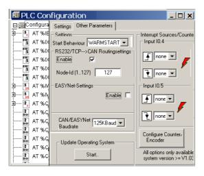
Figure 57:CAN Master routing settings
