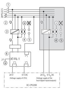
Figure 12:Example of wiring for power supply unit
