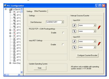
Figure 23:Updating the operating system of the XC-CPU201
