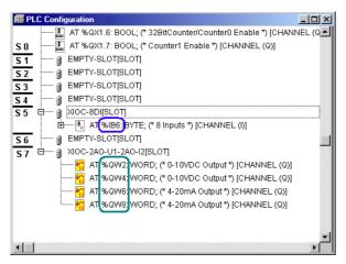
Figure 66:Configuration change through removal of the module (S0, S1, ..., S7 = slot number on rack)
