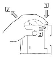
Figure 10:Detaching the modules
