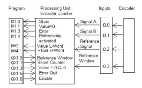
Figure 69:Inputs/outputs for incremental encoders
