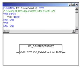
Figure 83: "IEC\_DeleteEventList" with declaration section function
