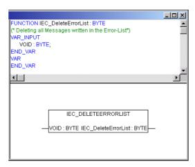
Figure 82: "IEC\_DeleteErrorList" with declaration section function
