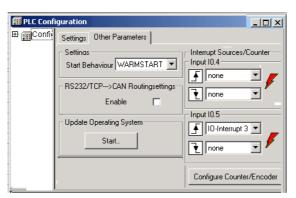
Figure 75: Allocation of I0.5 → interrupt source
