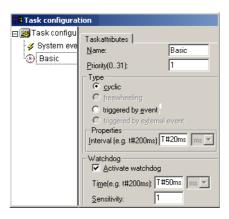
Figure 30:Parameterization of the cyclic task
