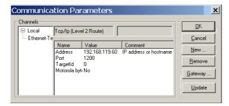
Figure 52: Communication parameters with IP address
