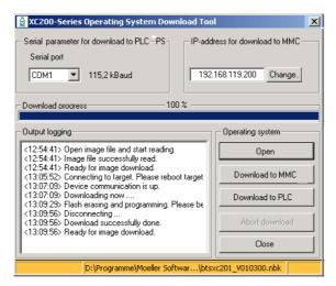
Figure 26:Download of the XC-CPU201 operating system ended
