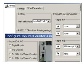
Figure 67:Incremental encoder preselection
