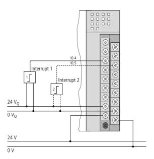
Figure 16:Interrupt input connections
