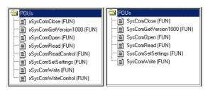
Figure 62:Overview of functions (left: xSysCom200.lib, right: SysLibCom.lib)
