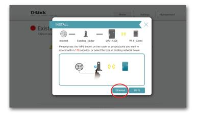
Connect an Ethernet cable to your DAP-1325 if you have not already done so. After making the connection, you will automatically be forwarded to the next step. If you haven't connected an Ethernet cable yet, but will do so later, click **Skip**.
