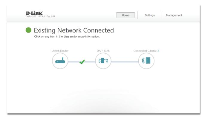
**Uplink Router:** This icon shows the status of the connection to the uplink router. It is grey if the DAP-1325 is not connected to an uplink router. Once connected, click on it to see its connection details.
