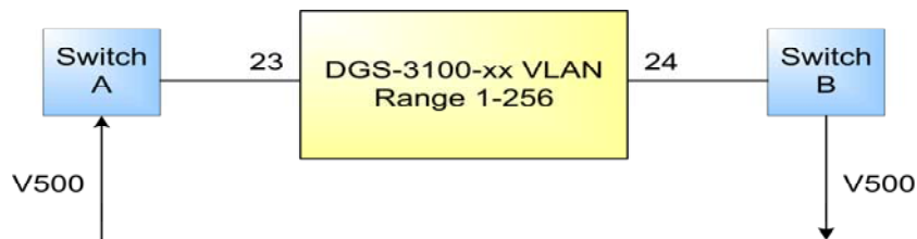
Figure 0–11. VLAN Trunking example between 2 switches
