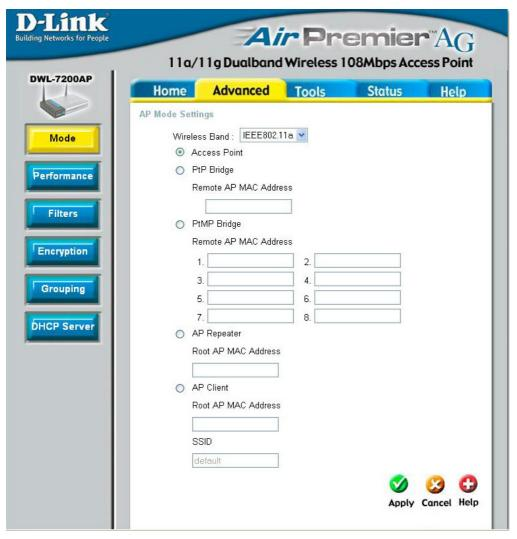
The DWL-7200AP can be configured to perform in any of five modes: Wireless Access Point, Wireless Bridge, Multi-Point Bridge, AP Client or Repeater.
