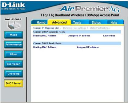
This screen displays information about the current DHCP dynamic and static IP address pools. This information is available when you enable the DHCP function of the DWL-7200AP and assign dynamic and static IP address pools.
