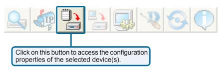
The device configuration window allows you to configure settings but does not actually apply the settings to the device unless you click the **Apply** button. You can also save and load configuration files from this window. When you load a configuration file, you must click **Apply** if you want the settings to be applied to the selected device(s).
