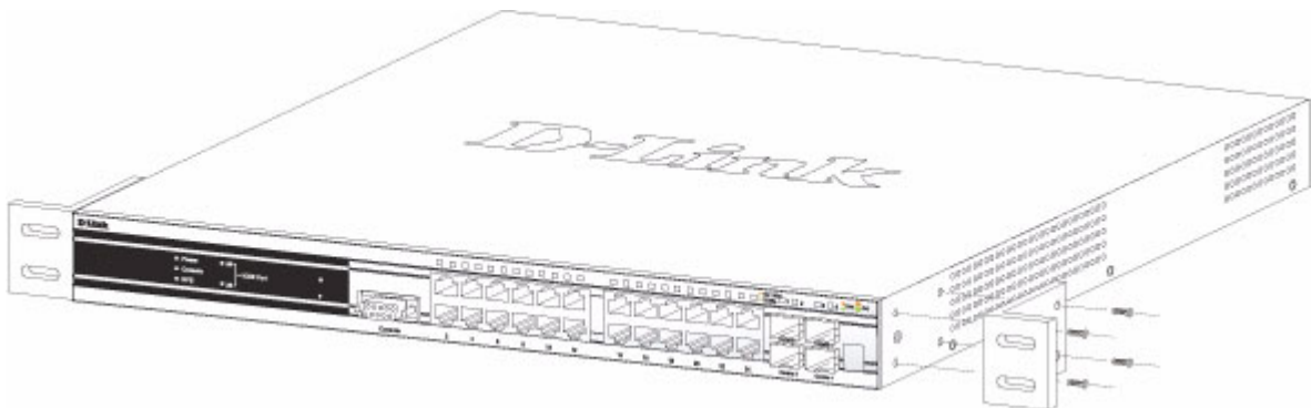
Figure 20. Fasten Mounting Brackets to Switch
