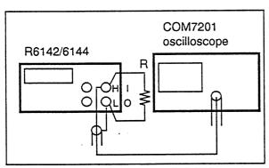
Figure 4-5 Cable Connection for Highfrequency Noise Voltage Measurement
