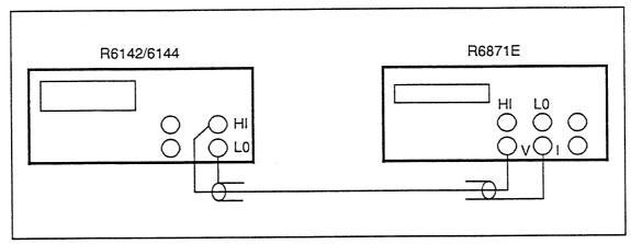
Figure 4-1 Cable Connection for Output Voltage Test
