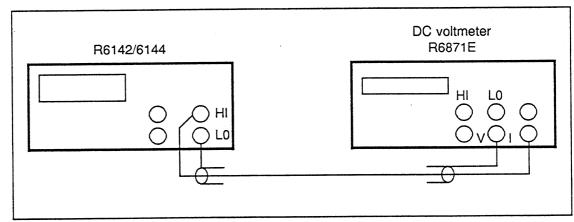
Figure 4-8 Cable Connection for Current Limiter Test
