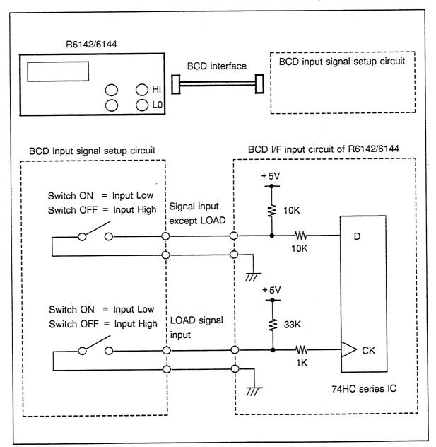
Figure 4-10 Cable Connection for BCD Interface Test
