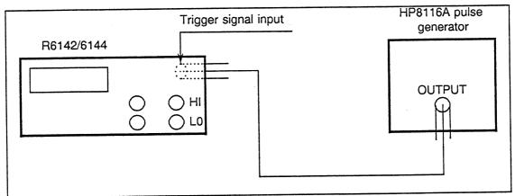
Figure 4-13 Cable Connection for Trigger Signal Test
