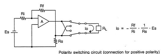
Figure 3-3 Principle of the Output Amplifier and Polarity Switching Circuit
