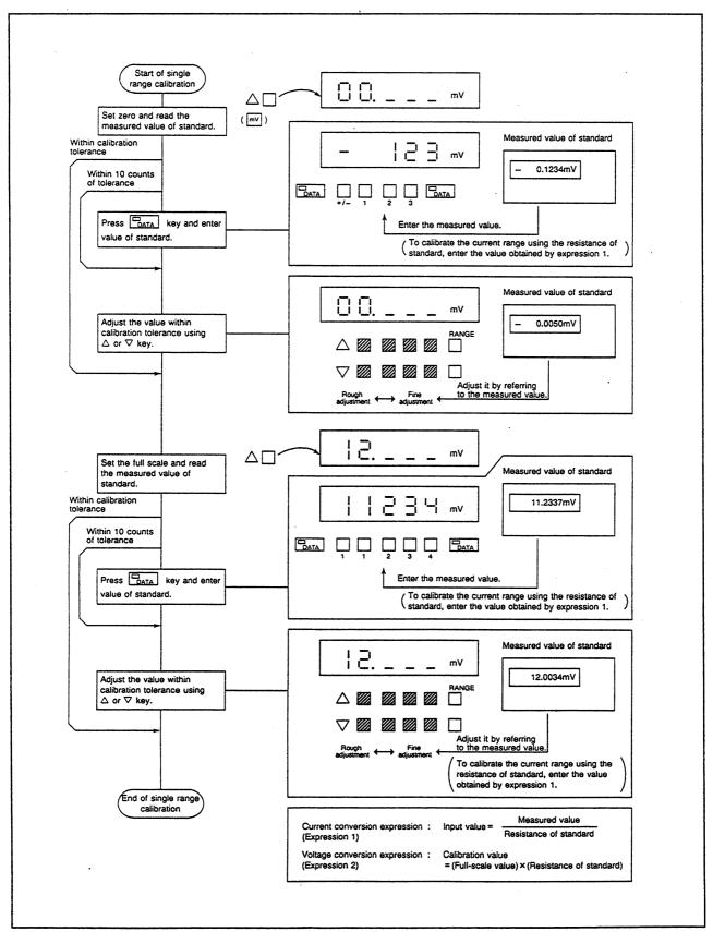
Figure 5-2 Calibration of A Single Range using R6142
