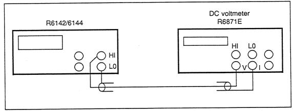
Figure 4-7 Cable Connection for Voltage Limiter Test
