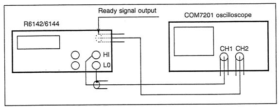
Figure 4-11 Cable Connection for Ready Signal Test
