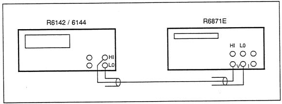
Figure 5-1 Cable Connection for Output Voltage Calibration
