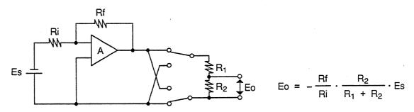
Polarity switching circuit (connection for positive polarity)
