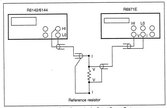
Figure 4-2 Cable Connection for Output Current Test
