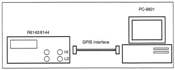
Figure 4-9 Cable Connection for GPIB Interface Test
