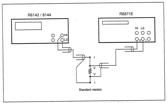
Figure 5-4 Cable Connection for Output Current Calibration
