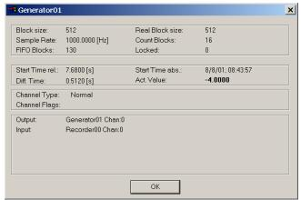
Press the Control key and click on the data line with left mouse button to display the status of the data channel during measurement.
