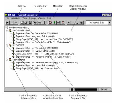
To control a multi-step application consisting of more than one DASYLab worksheets calling each other, DASYLab offers a new tool, shown as new display window (analogous to the worksheet, display and VITool windows), called the Control Sequencer Window. The contents of the window is stored in a new type of file, the Control Sequencer file (saved with the suffix \*.DSQ.)
