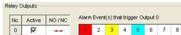
Output Relay 0, Active, Normally Closed – Shown set to Open on Alarm Conditions on Channels 1, 3, or 5
