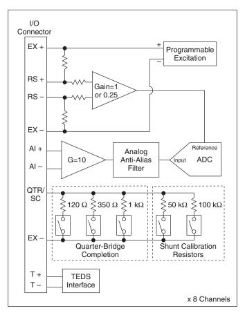
Figure 2-18. NI PXIe-4330/4331 Signal Conditioning Block Diagram
