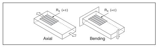
Figure 2-3. Quarter-Bridge Type I Measuring Axial and Bending Strain
