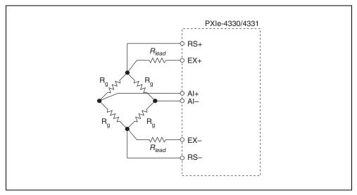
Figure 2-2. Connecting Remote Sense Wires to the NI PXIe-4330/4331
