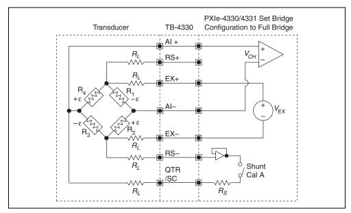
Figure 2-12. Full-Bridge Type I Circuit Diagram
