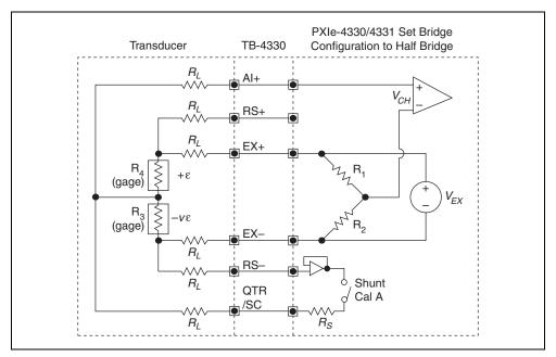
Figure 2-8. Half-Bridge Type I Circuit Diagram
