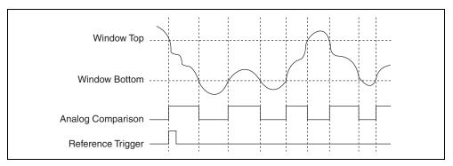
Figure 2-23. Window Triggering
