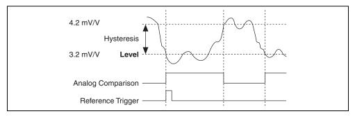
Figure 2-22. Analog Edge Triggering with Hysteresis on Falling Slope
