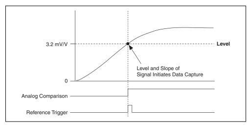
Figure 2-20. Analog Level Trigger on Rising Slope
