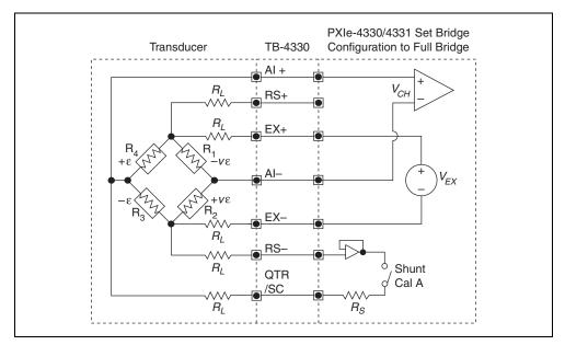
Figure 2-14. Full-Bridge Type II Circuit Diagram
