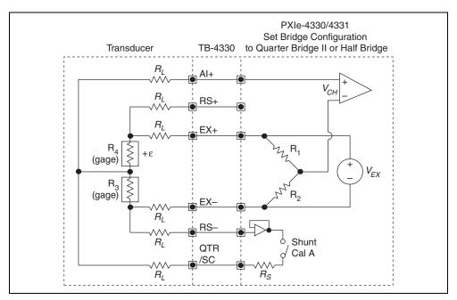
Figure 2-6. Quarter-Bridge II Circuit Diagram
