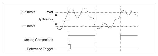
Figure 2-21. Analog Edge Triggering with Hysteresis on Rising Slope
