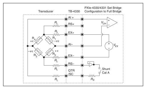
Figure 2-16. Full-Bridge Type III Circuit Diagram
