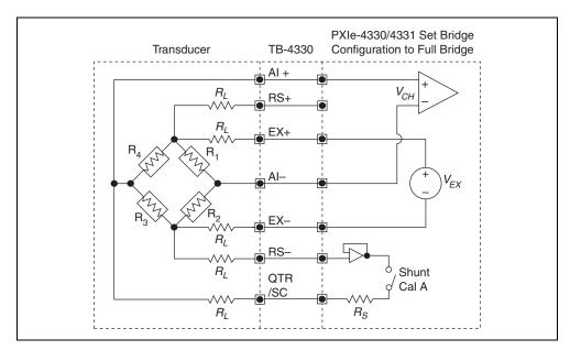
Figure 2-17. Force, Pressure, and Torque Sensor Circuit Diagram
