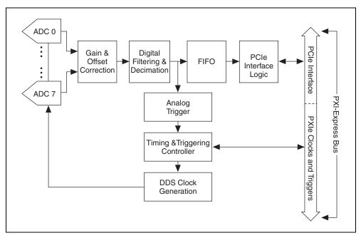
Figure 2-19. NI PXIe-4330/4331 Digital Back End Block Diagram
