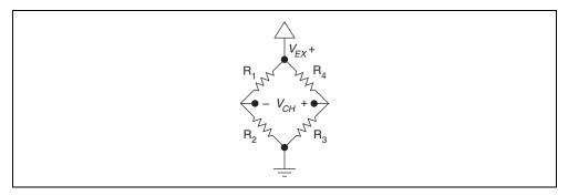
Figure 2-1. Basic Wheatstone Bridge Circuit Diagram
