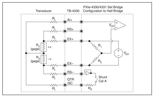
Figure 2-10. Half-Bridge Type II Circuit Diagram
