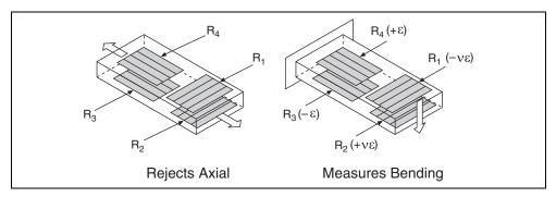
Figure 2-13. Full-Bridge Type II Rejecting Axial and Measuring Bending Strain
