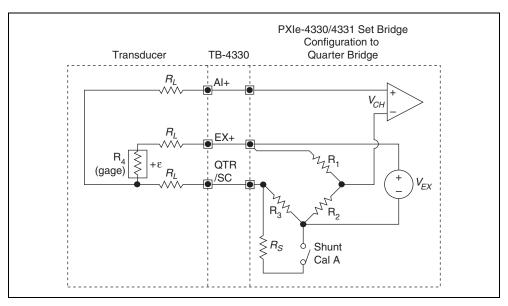
• Sensitivity ~  $0.5 \,\mu\text{V/V}$  per  $\mu\epsilon$ , for GF = 2.0.
