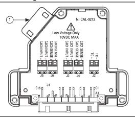
1 Ground Lug (on the bottom side of the NI CAL-9212 enclosure)
