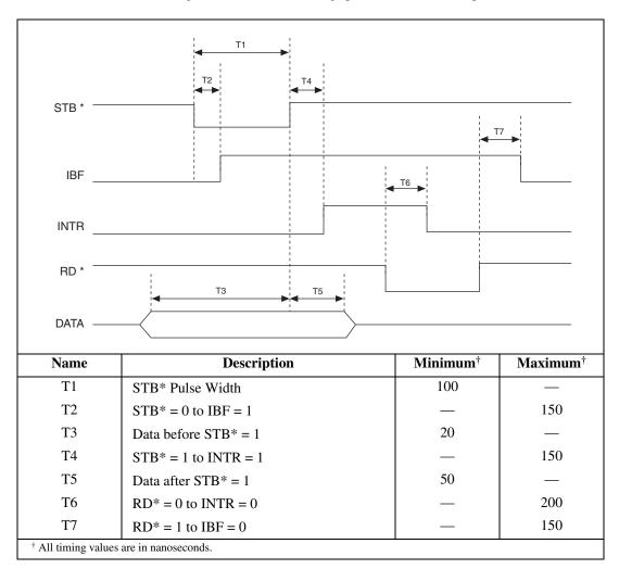
Figure 4-2. Timing Specifications for Mode 1 Input Transfer
