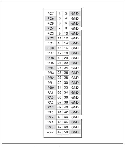
Figure 3-3. PCI-6503 I/O Connector Pin Assignments
