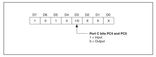
Figure B-7. Control Word to Configure Port A for Mode 1 Output
