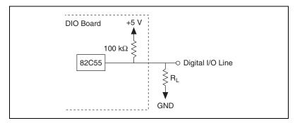
Figure 3-5. DIO Channel Configured for High DIO Power-up State with External Load
