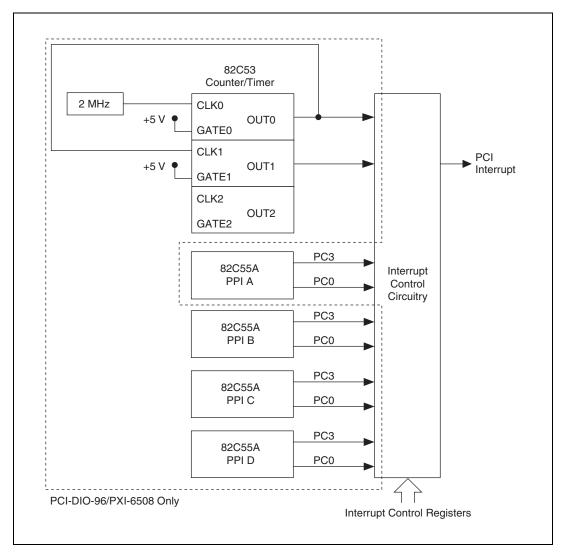
Figure B-1. Interrupt Control Circuitry Block Diagram
