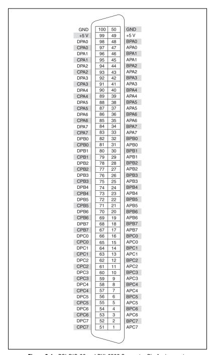
Figure 3-1. PCI-DIO-96 and PXI-6508 Connector Pin Assignments
