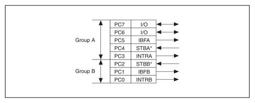
Figure B-6. Port C Pin Assignments on I/O Connector when Port C Configured for Mode 1 Input
