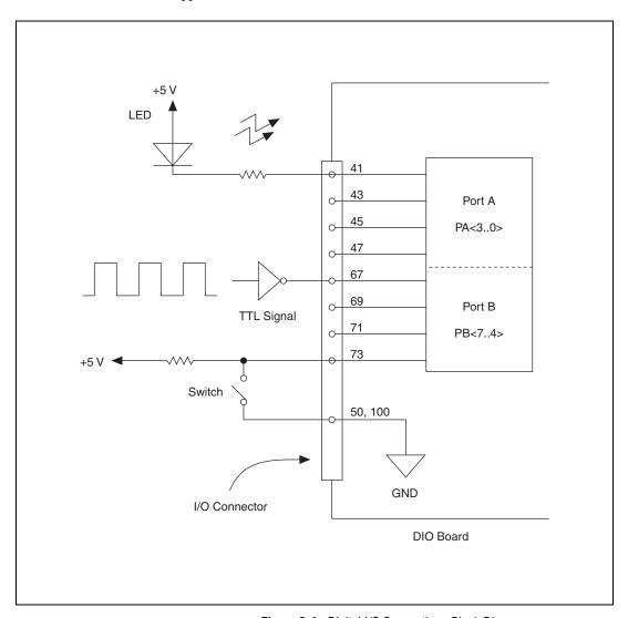
Figure 3-4. Digital I/O Connections Block Diagram
