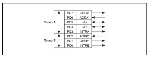
Figure B-9. Port C Pin Assignments on I/O Connector when Port C Configured for Mode 1 Output
