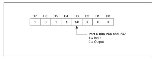
Figure B-4. Control Word to Configure Port A for Mode 1 Input
