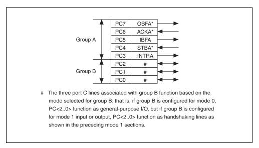
Figure B-11. Port C Pin Assignments on I/O Connector when Port C is Configured for Mode 2
