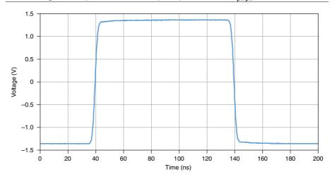
Figure 7. Square Waveform Step Response at 12  $V_{pk\text{-}pk}$ , Measured
