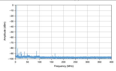
At amplitude of -1 dBFS and measured from DC to the sixth harmonic.
