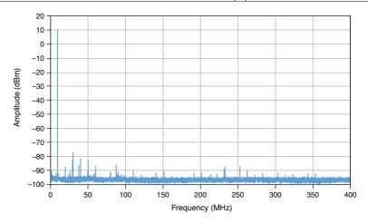
Figure 4. 1 MHz Spectrum  $^{15}$  at 6.5  $V_{pk-pk}$ , Measured
