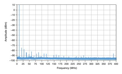
$<sup>^{24}</sup>$  Relative to 50 kHz and at 2  $V_{pk\text{-}pk}$  and maximum user sample rate.  $^{25}$  With the digital filter enabled and at -1 dBFS, 2  $V_{pk\text{-}pk}$ , and 400 MS/s. Noise floor is limited by the noise floor of the measurement device.
