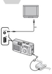
Connecting the camera to a TV via the supplied video cable ①, it is possible to view and playback the recorded images.
