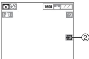
When the flash/access indicator ① and card access indication ② light, do not:
