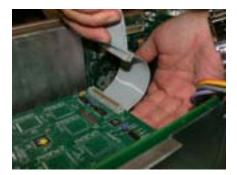
Figure 5: Attaching Ribbon Cable to HD DSP board
