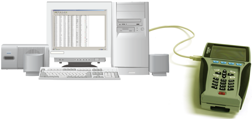
Figure 7.1 Diagram of Validator-NT Connected to PC
