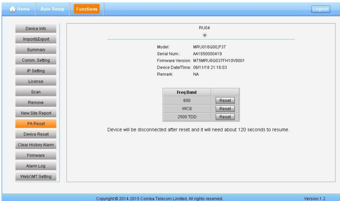
Figure 58: Function - PA Reset
