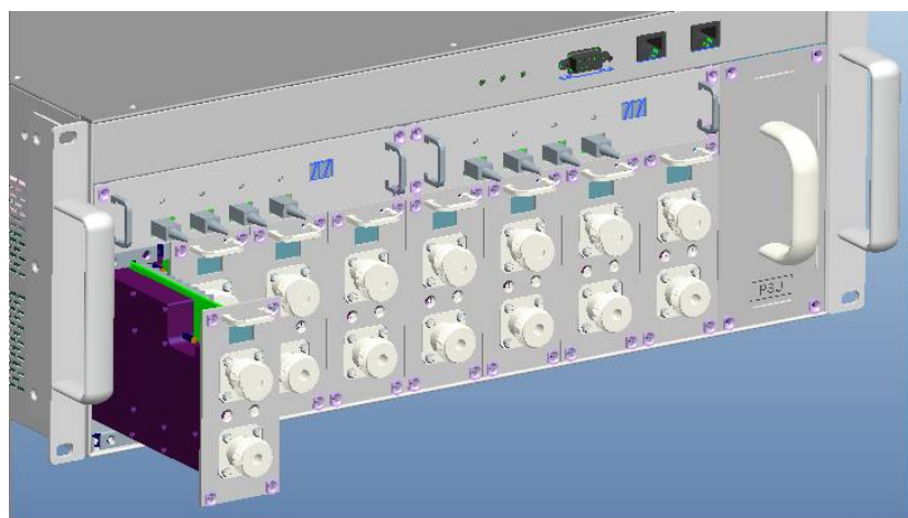
Figure 6: RF Unit Installation
