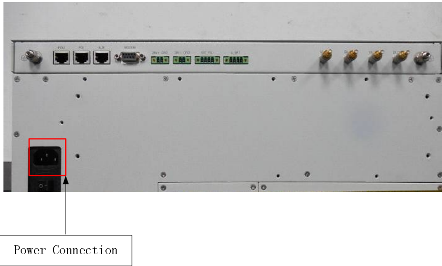
Figure 30: MU Power Connection (Rear Panel)
