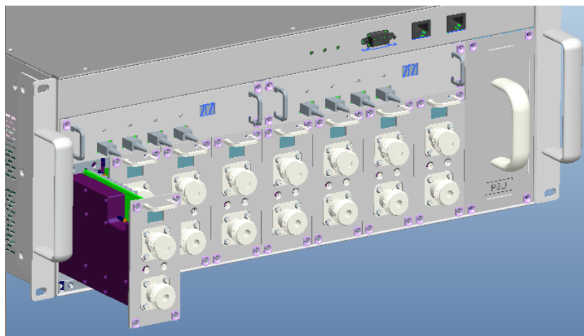
Figure 6: RF Unit Installation
