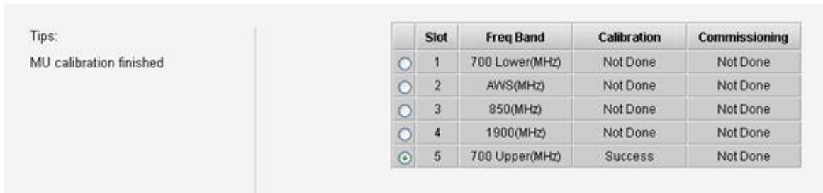
Figure 68: Commissioning Procedure – MU Calibration Finish
