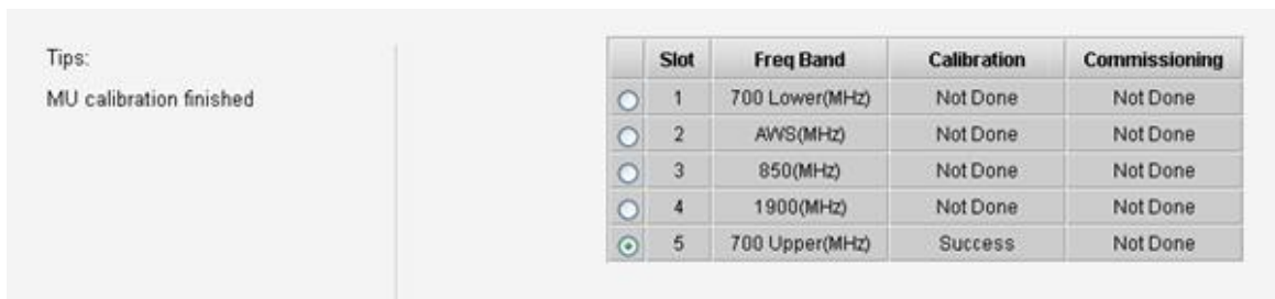
Figure 74: Commissioning Procedure – MU Calibration Finish
