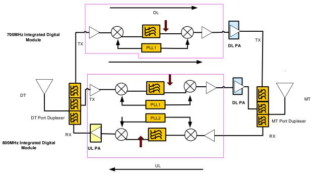
Figure 2: PS BDA Functional Block Diagram
