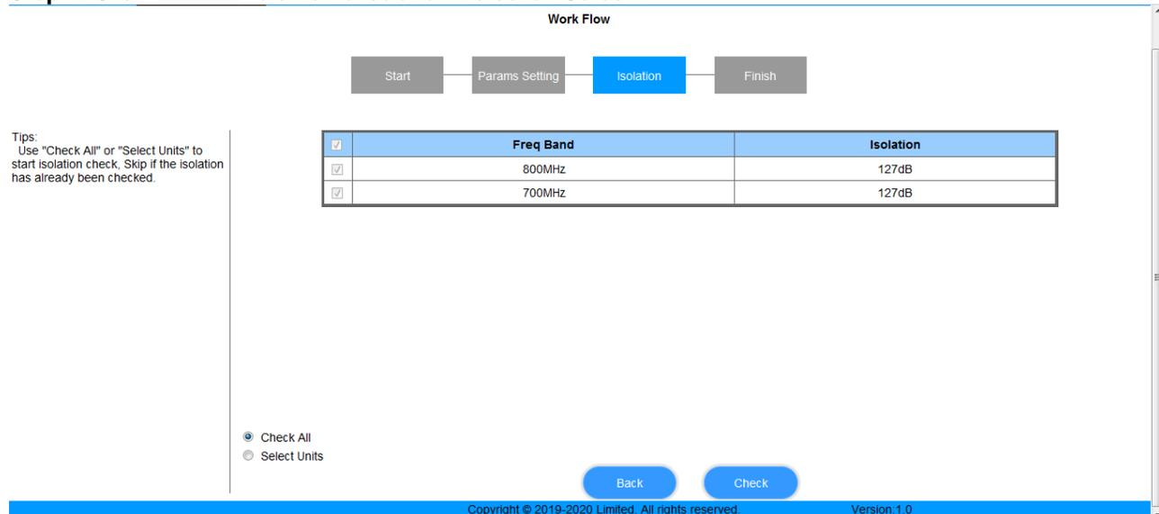
Figure 30: Commissioning Procedure – Isolation Detection
