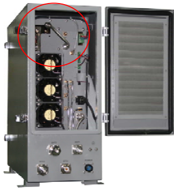
Figure 8: Attach MCPA Unit in Back Panel
