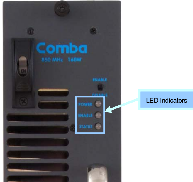
Figure 1: Controls and Indicators on Front Panel of MCPA Module
