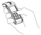
Select the directional or omni-directional microphone with the arrow buttons in the middle (see page 12). Place the receiver on a table or aim it at the person you want to listen to. Choose directional or omni-directional settings depending on the situation. Normally in noisy surroundings directional setting is preferred.
