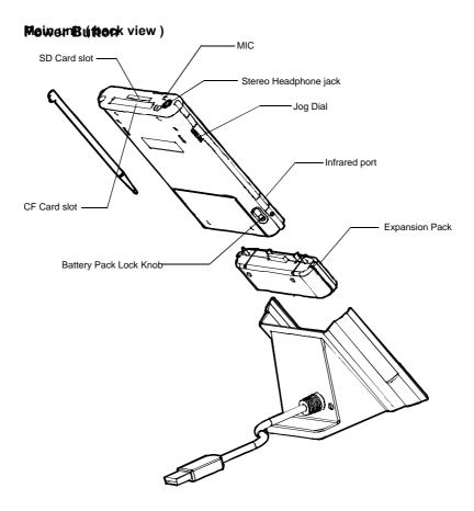
The power button turns the unit and the front light on and off.
