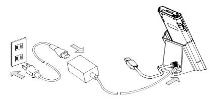
2. Connect the supplied AC adapter and the Toshiba Pocket PC as shown in the figure below.
