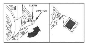
**NOTE:** When adding oil to the engine crankcase, use a high quality detergent oil classified "For Service SF,SG,SH" rated SAE 30 weight. Use no special additives. Select the oil's viscosity grade according to your expected operating temperatures.
