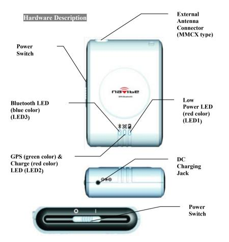
The Bluetooth GPS has three LED indicators. The first is low power LED indicator that is named LED1. The second is GPS & Charge status LED that is named LED 2. The third is Bluetooth status LED that is named LED 3. The status table of LED shows as follows:
