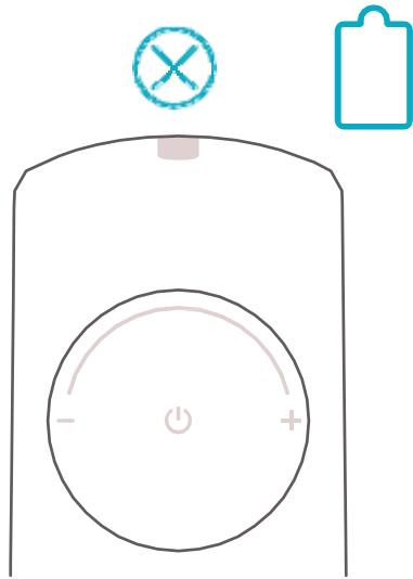
The charging cable is inserted into the charging socket, and the status indicator lamp shows orange light, which means the product enters into the state of charging.
