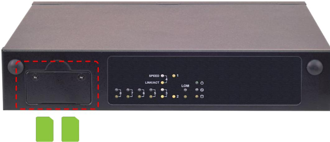
1. Loosen the two screws that secure the SIM slot cover and remove the slot cover. With the angled corner facing inward, push the SIM card all the way in until it clicks into place.
