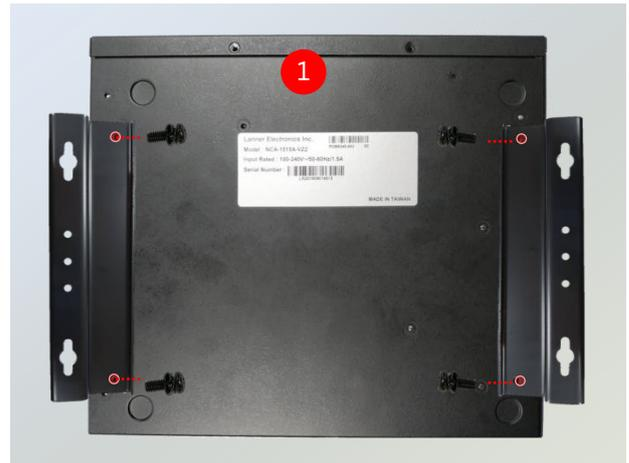
2. On the wall, measure the exact place where you want to hang the system and drill four holes.
