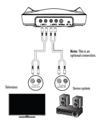
Note: If your audio device does not have RCA outputs, you can use the 3.5 mm-to-RCA adapter (included) to make the connection Your setup may differ from the example shown here.
