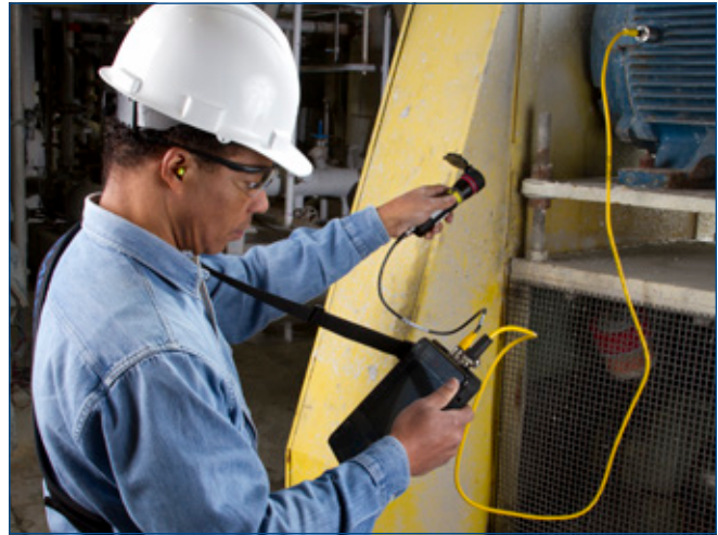
The CSI 430 Laser Speed Sensor determines shaft speed without shutting down the machine - even in extremely tight locations.
