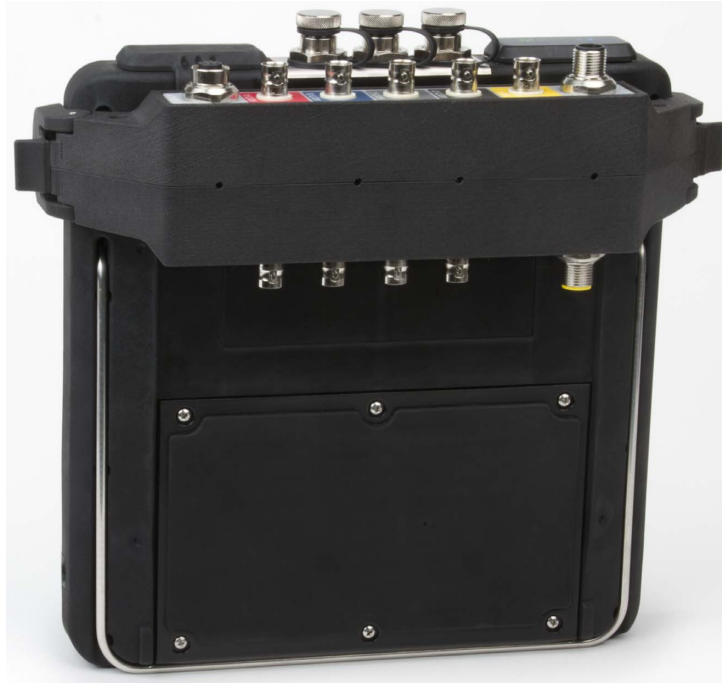
Figure 2-13: CSI 2140 Four-Channel Input Adapter attached to the CSI 2140 without the interface cable
