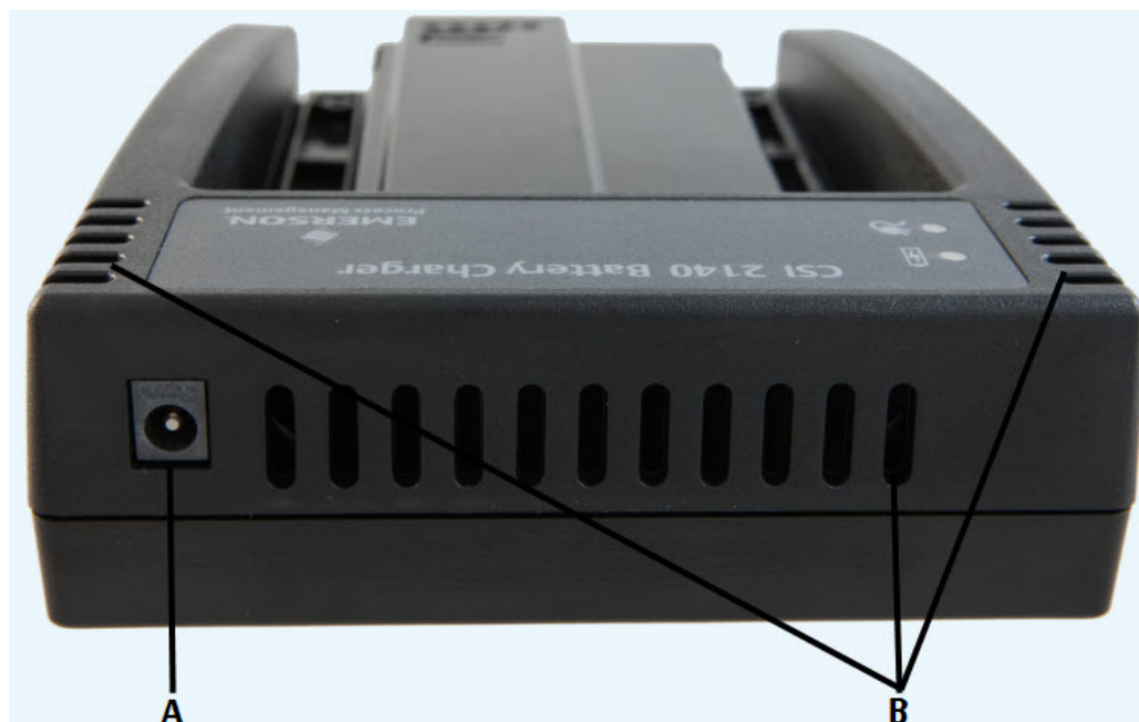
Figure 2-6: Power supply connector and air vents
